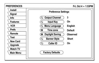
**Set output channel** Use the *Output Channel* menu button to toggle between channels 3 and 4, whichever is unused in your area.
